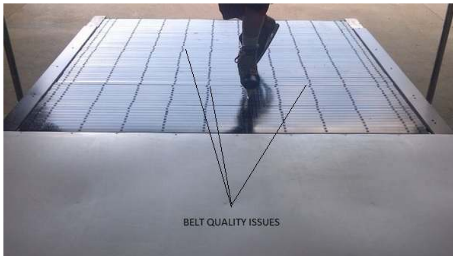
Competitor's Belt is Bumpy and misaligned
