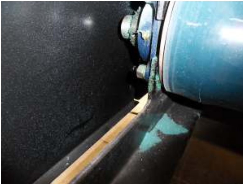
Competitor's treadmill shown with belt dust on frame.
